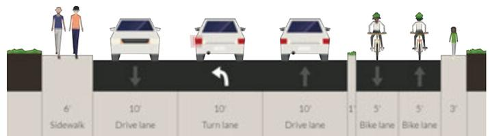
Cross section of Route 135 showing left turn lane and Option 2 with one two-way separated bike lane.
